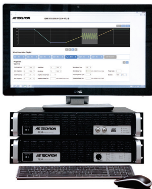
The 3110 Waveform Generator and a 7224 amplifier form the basic SWG System
